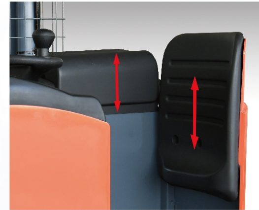
Adjustable backrest and armrest help reduce fatigue
